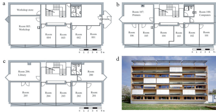
Fig. 1. LESO-PB building: (a) ground floor; (b) first floor; (c) second floor; (d) southern façade.
