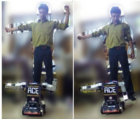
Figure7. Imitation of its human operator by ACE, the semi-humanoid robot.
